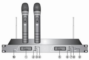
(1) (5)LCD: when power is on, it becomes green which can show FREQ (receiving frequency of the device);00~30 (rate of sound volume).Line A/B (channel A or B); \(\nabla\) (radio frequency indicator) which shows the level of the signal when the microphone is on."))))" (acoustical frequency level indicator) it waves with the sound of microphone, from 0dB-35dB to " " "
